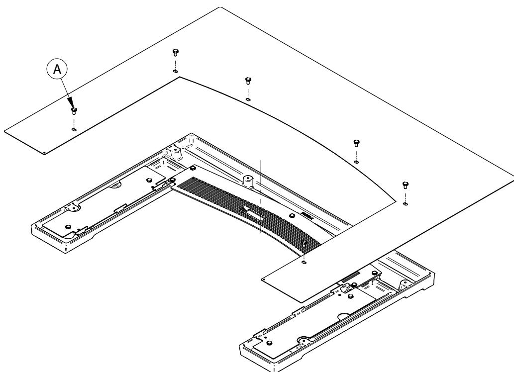
3. Align the faceplate hooks with the insert and slide the faceplate down to hook it on the insert.
