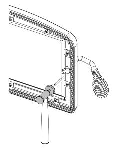
Figure 11: Installing the split pin
