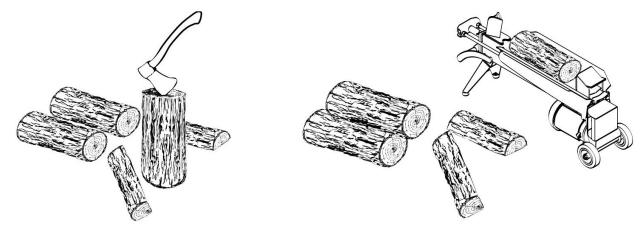
Wood should be split to a range of sizes, from about 75 mm to 150 mm (3" to 6") in cross section. Having a range of sizes makes starting and rekindling fires much easier. Often, the firewood purchased from commercial suppliers is not split finely enough for convenient stoking. It is sometimes advisable to resplit the wood before stacking to dry.
