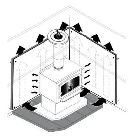
Figure 13: Heat shield
