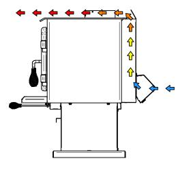
Figure 7: Air flow with a blower
