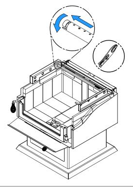
Note that secondary air tubes (B) can be replaced without removing the baffle board (A) and that all tubes are identical.
