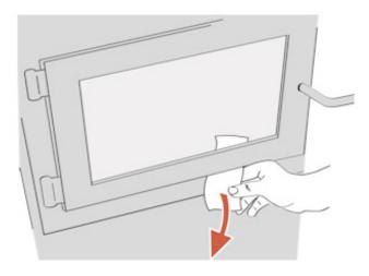
Figure 9: Door gasket seal verification
