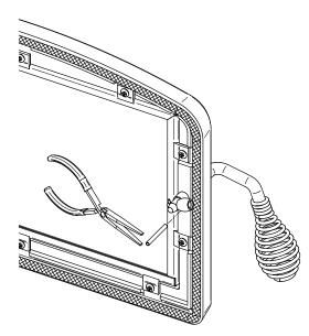
Figure 10: Removing the split pin
