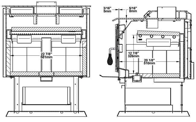
Figure 5: Front view - Combustion chamber
