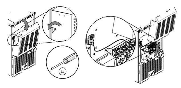
2. Use the screws (B) to secure the battery holders (A) on the stove's back panel.
