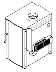
When using the blower, allow the wood fire to reach operating temperature (approximately one hour), before turning it on. The increased airflow from the blower cools the firebox and could affect the start-up combustion efficiency if the blower is turned on too early.
