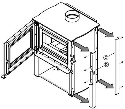
3. Unscrew and remove the pillar (C) and (D).
