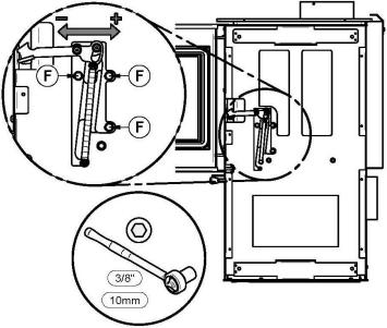
To adjust door tightness, slightly loosen the bolts (F). The more distant from the door is the mechanism, the stronger the tightening will be.
