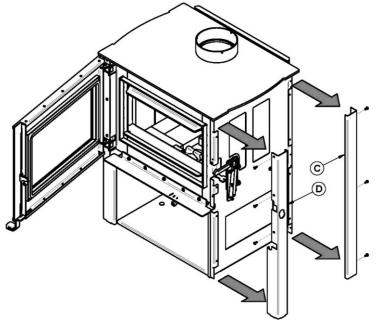
3. Unscrew and remove the pillars (C) and (D).
