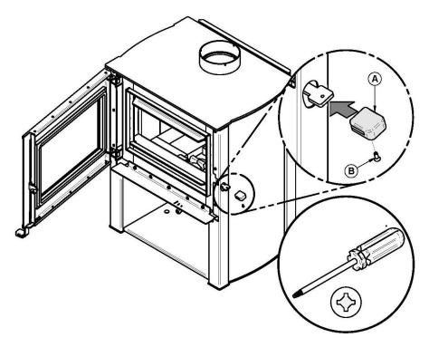
6. Reinstall the handle (A) with the screw (B)
