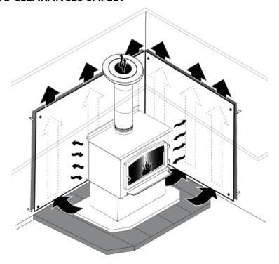
Following the installation of such heat radiation shields, the minimum clearances to heat-sensitive materials may be reduced by applying the clearances factor in the table below:
