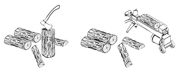
Wood should be split to a range of sizes, from about 75 mm to 150 mm in cross section. Having a range of sizes makes starting and rekindling fires much easier. Often, the firewood purchased from commercial suppliers is not split finely enough for convenient stoking. It is sometimes advisable to resplit the wood before stacking to dry.
