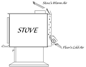
CAUTION: ENSURE THAT THE BLOWER'S POWER CORD IS NOT IN CONTACT WITH ANY SURFACE OF THE WOOD FIRE TO PREVENT ELECTRICAL SHOCK OR FIRE DAMAGE. DO NOT RUN THE POWER CORD BENEATH THE WOOD FIRE.
