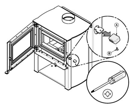
2. Unscrew screw (B) and remove the handle (A).
