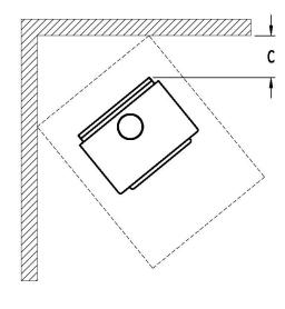
Clearances to heat-sensitive materials and floor protection
